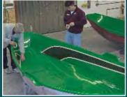
Every ClackaCraft is built on a carefully-designed mold. Fiberglass and fiberglass material are applied *inside* the mold in layers. Every layer is done by hand by skilled craftsmen. The accent color is placed, then the bottom is laid. The chine area is built up to make the superstrong chines ClackaCraft is famous for. Side material is added. Last, interior components are added to the hull.
